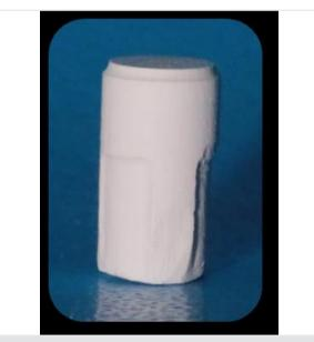
Figure 1. Side view of zirconia sample produced with CAM
