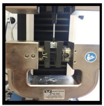
**Figure 3.** Instron universal test device and a sample put into the device
