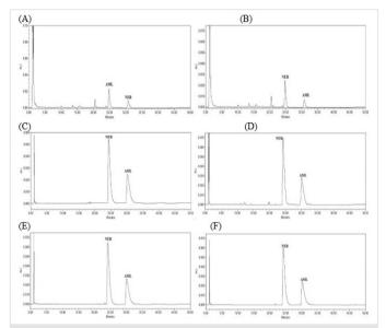
**Figure 3.** Chromatograms of AML and NEB at synthetic mixture (A) acid-degraded drug, (B) base-degraded drug, (C) water hydrolysis-degraded drug, (D) oxidation-degraded drug, (E) thermal-degraded drug and (F) daylight-degraded drug
